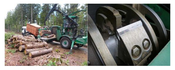
Figure 1: Chipping with the self-propelled Albach Diamant 2000 (left) was carried out with new and sharp knifes (right)
