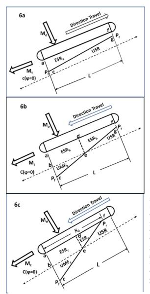
Fig 6. Diagrams illustrating the three scenarios for the track pressure-soil resistance  $c(\phi=0)$  interface
