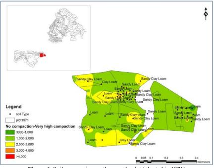
Figure 6 Soil compaction on the sample plot (planted in 1971)
