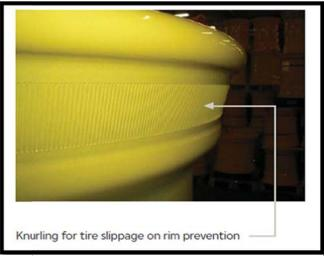
not painted. A slipping wheel on the rim will destroy the tube by tearing off the inflation valve. Even in the tubeless version, intense wheel slip will wear out the contact area of the tyre bead and therefore further reduce the torque transmitted between rim and tyre.
