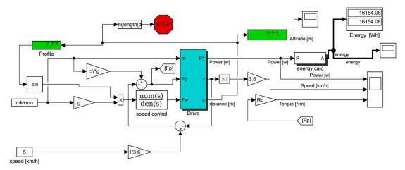
Fig. 2 A basic model of the trailer's electrical drive realized in MATLAB/Simulink.
