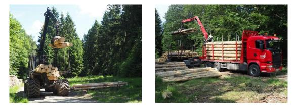
Figure 4: Forwarding and transporting debarked logs, within a field trial in central Germany
