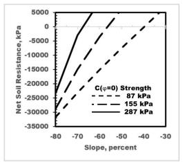
Fig 7. Net soil resistance is dependent on the  $c(\phi=0)$  value of soil strength and slope when traveling downslope. Negatives values are indicative of a sliding failure.
