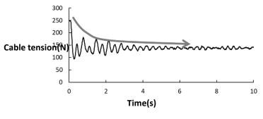
Figure 2 Tension damping
