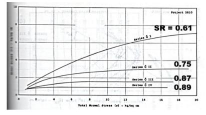
Fig 2. Failure curves as a function of  $\tau$  (y axis) and  $\sigma$  (horizontal axis) for wet, partly saturated soils at four saturation ratios (Casagrande and Hirschfeld 1960)
