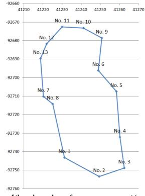
Figure 3. Illustration of the polygonal area for area measurement (coordinate: Japan Plane Rectangular Coordinate System Zone III; unit: m)
