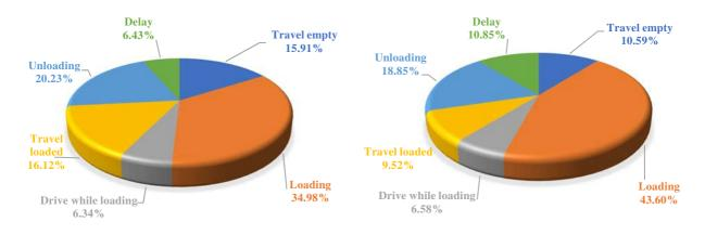
Fig. 4 - Site A forwarder work elements distribution
