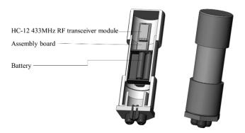
Figure 3 3D model of the Control unit
