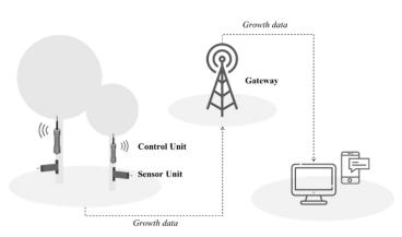
Figure 5 Working principle of prototype tree growth monitoring device
