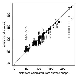
Figure 5 Measured and calculated distances between actual cutting slopes and the sensor
