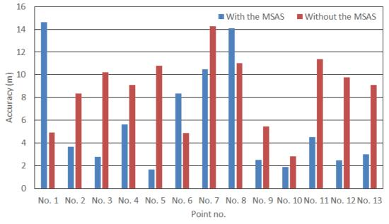
Figure 6. Summary results of GNSS measurements at the 13 vertex points
