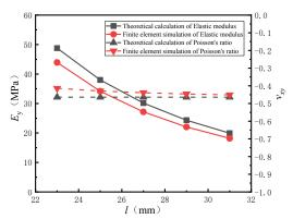
Fig. 10 The influence of cell half-width *l* on in-plane elastic constants with topological density of  $\lambda_2$
