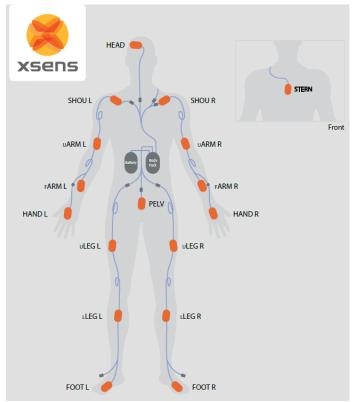
Figure 4. Positions of IMU sensors on human body
