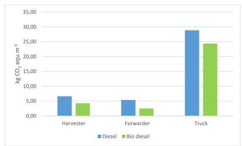
Figure 4: Effects of the transition from diesel to bio diesel on the global warming potential of harvester, forwarder and truck
