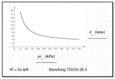
ing the wheel performance depending on the inflation pressure. The WES-method was developed in the Waterways Experiment Station in Vicksburg, Mississippi, a United States Army Corps of Engineers research facility. It is based on semi-empiric modelling of wheel performance and on measuring soil penetration resistance by a standardized cone penetrometer.
