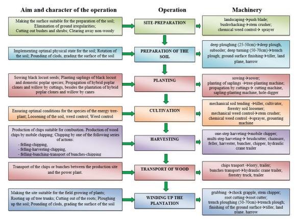
Figure 3. Operations and machines of energy tree plantation technologies (based on Czupy et al., 2012)
