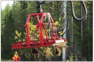
Fig 1. Naarva P25 -device for mechanized PCT by uprooting.
