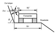
Figure 1 Parameters of logging roads and a forwarder
