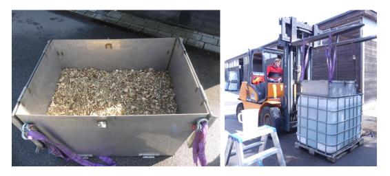
Figure 2: Washing woodchips; left: washing box with FRC; right: lifting the washing box into and out of the IBC tank;
