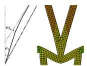
Fig. 8 Large deformation diagram of honeycomb long wall with topological density of  $\lambda_1$
