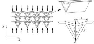
Fig. 3 The parameters of the cell of the V-winged NPR honeycomb
