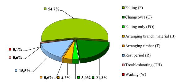
Figure 3.: Working day structure of Ponsse Ergo 6WD harvester (Rátky, 2019)
