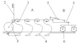
Fig. 2 General scheme of a vibro-combinator (Caproiu St. et al, 1982; Biris S.St. et al, 2015)
