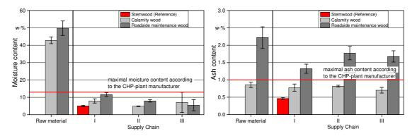
Figure 5: Left: Moisture content (in w-%) for the raw materials and after processing with the three supply chains and the maximal recommended moisture content (mean values ± standard deviations). <u>Right:</u> Ash content (in w-%, dry basis) for the raw materials and after processing with the three supply chains (mean values ± standard deviations) and the maximal recommended ash content
