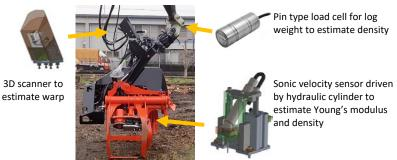
Figure 3. New harvester head with 3D scanner and sonic velocity sensors
