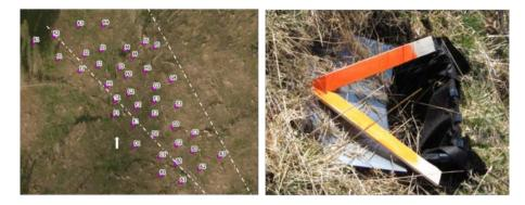
Figure 1 Layout of the sediment traps on the 60% hillslope. The dashed lines show the position of the cable corridors while the arrow indicates the downhill direction (left). Close-up of sediment trap after 2 years, the orange marker indicating the position of ground control point used in processing UAV imagery
