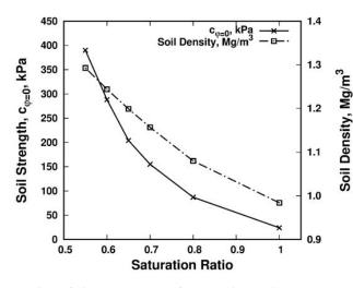
Fig 5. Soil strength,  $c\phi=0$ , and soil density as a function of the saturation ratio
