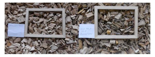
Figure 6: Left: Reference wood chips (stemwood of Norway spruce) after processing in supply chain I (size of the rectangular frame = DIN A5). Right: Roadside maintenance wood chips upgraded in supply chain I (size of the rectangular frame = DIN A5)
