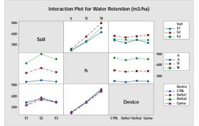
Fig. 10 Interval plot for water retention (from three-way ANOVA) for soil types (factor Soil), depth (factor h) and active elements (factor Device).
