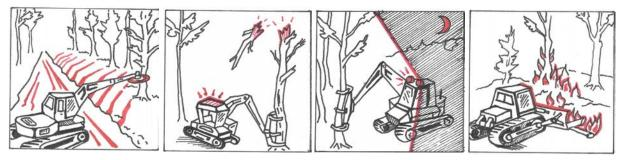
Figure 3 - Safety advantages using mechanized wildfire operations: cut, position, night operations, clear hotspots Graphics credit: Ry Basko
