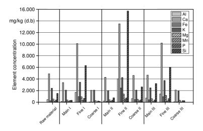
Figure 8: Element analyses of roadside maintenance wood for the three supply chains
