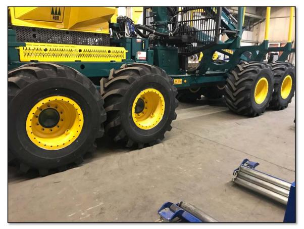
Fig 7: Test forwarder with bead-lock rims
