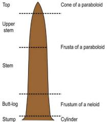
Figure 2 Stem parts with recommended geometrical 3D shapes for volume assessment (Husch et al. 2003) Given the same basic inputs (diameter, length and wood defects) are used in different scaling methods, one would assume that there is a good level of uniformity and harmonisation of methods; unfortunately, this is not often the case (Fonseca 2005). Most commonly used equations for volume determination are (Fonseca 2005, Sertié 2012):
