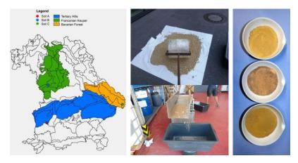
Figure 1: Left: Location of three different soil types. Each soil is representative for the considerable parts of the region (Zimmermann; 2019); centre top: crushing with a concrete roller; center bottom: screening at 2 mm with a self-constructed vibration screen; right, from top to bottom: soils A, B and C;
