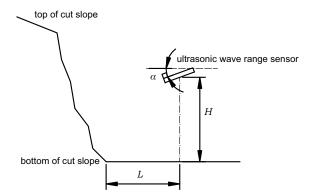
Figure 3 Experiment on ranging accuracy of actual cutting slope
