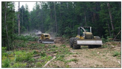
Image 1 - Cutting indirect fireline with feller-buncher, while track and wheel skidders swing logs to decking area
