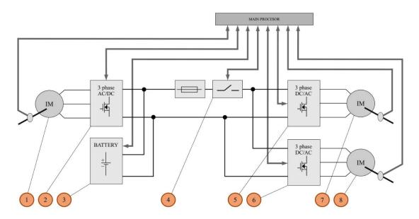
Fig. 1 Block diagram of the hybrid trailer drive
