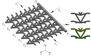
Fig. 4 Finite element simulation and boundary conditions
