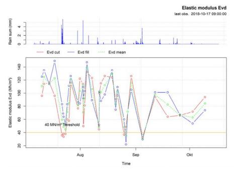
Figure 1. Recorded rainfall, elastic modulus on both lanes including the mean and threshold of 40 MN/m<sup>2</sup> plotted over time after Fritz (2018)
