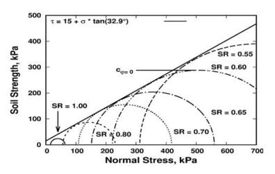
Fig 3. The  $c(\phi=0)$  values of soil strength for an essentially saturated soil compressed at a initial SR between 0.55 and 1
