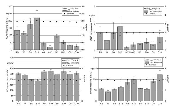
Figure 5: Combustion trials; left top: CO emissions; right top: Org.-C emissions; left bottom: NOx emissions; right bottom: total particle matter (TPM) emissions. Whiskers indicate the range of minimal and maximal values for the measurements. STC = standard test conditions.
