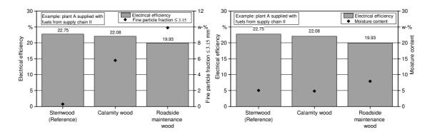
Figure 10: Left: Electrical efficiency (in %) of Plant A in relation to fine particle fraction (≤ 3.15 mm in w-%) for fuels processed with supply chain II. <u>Right:</u> Electrical efficiency (in %) of Plant A in relation to moisture content (w-%) of fuels processed in supply chain II
