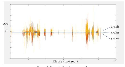
Figure 3. Record of chainsaw operation. t: 1.5-3.0\*10<sup>5</sup>: felling, 3.5-5.0\*10<sup>5</sup>: cross cutting, 8.2-9.0\*10<sup>5</sup>: delimbing blue: x-axis, red: y-axis, yellow: z-axis
