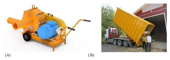
Figure 2: Small-sized blower (A) and container truck with a blower attached at the back (B) (Föhr, KC, Karhunen Laihanen and Ranta, 2019)
