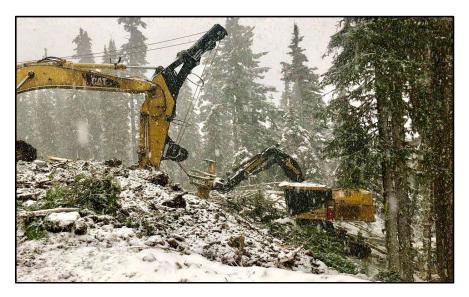
Figure 4. Tractionline winch-assist and Tigercat L870C feller buncher: Case Study 4
