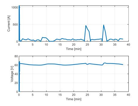
Fig. 4 - Simulated data of the battery current and voltage during the trailer operation cycle
