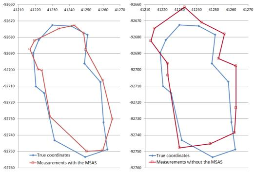
Figure 7. Results of area measurements with and without the MSAS correction (left: with the MSAS correction; right: without the MSAS correction)
