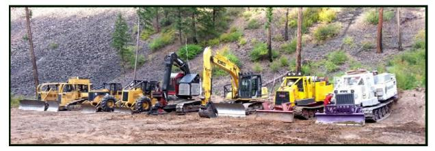
Image 2 - Left to Right: Dozer, pumpercat, wheel skidder, wheel skidder with drop-tank, feller-buncher, excavator, softtrack skidgines
