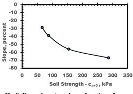
Fig 8. Downslope travel as a function of  $c(\phi=0)$  when a sliding failure is anticipated
