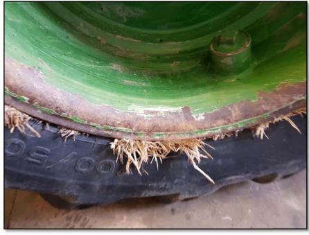
branches can slide between the rim flange and the tyre, see Fig. 6. Especially wooden splinters can be pressed with high forces against the rim flanges when the wheel is side sliding against a tree stump. With tubeless mounted wheels,
