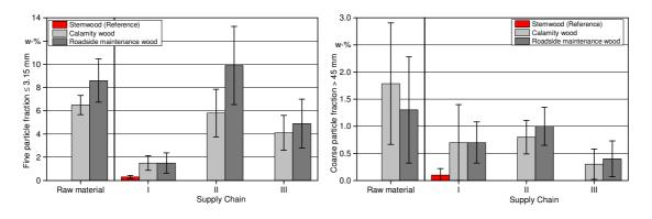
Figure 7: Left: Fine particle fraction (≤ 3.15 mm) in w-% for the raw materials and after processing with the three supply chains (mean values ± standard deviations). <u>Right:</u> Coarse particle fraction (> 45 mm) in w-% for the raw materials and after processing with the three supply chains (mean values ± standard deviations)
