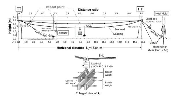
Figure 1 Schematic diagram of the experimental line
