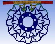
Fig. 11 The deformation of feeding rollers under an average pressure like the weight of an Eucalyptus
