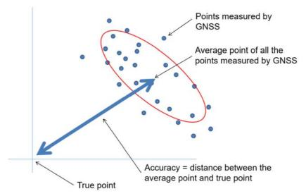
Figure 4. Definition of accuracy and its calculation
