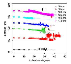
Figure 4 Measured and calculated distances between the tilted flat board and sensor
